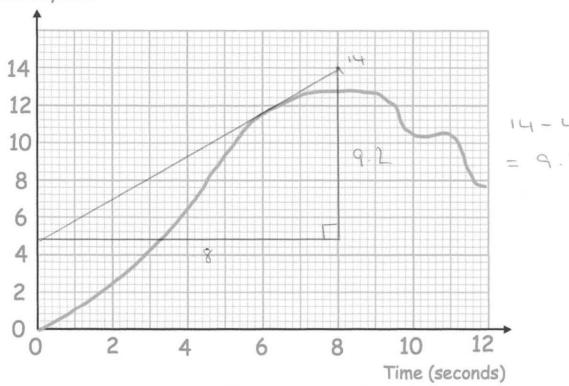
Above is the velocity-time graph of a particle over 12 seconds.
